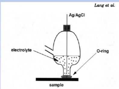
Figure 2. Diagram of the measurement cell for the electrochemical experiments.
