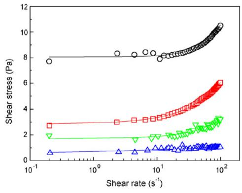
Fig. 6. A plot of shear stress as a function of shear rate for 30/70 hexane/water emulsions prepared with ( $\triangle$ ) 1%; ( $\nabla$ ) 2%; ( $\square$ ) 3% and ( $\bigcirc$ ) 5% bentonite, 0.01% CTAB, and 0.01 M NaCl. The solid lines are the lines of best fit to the Herschel–Bulkeley mode 1 [37].
