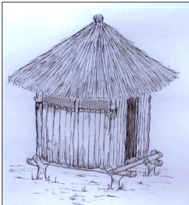
An aerated storeroom
